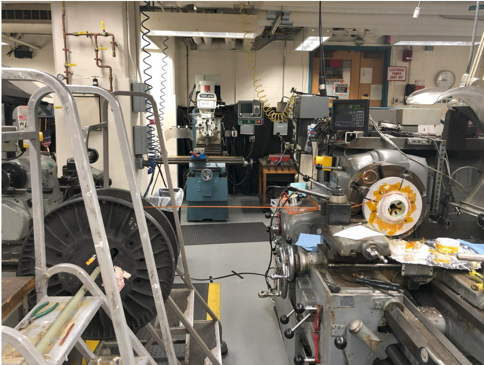
Figure A.2: The coil winding setup on the lathe.
