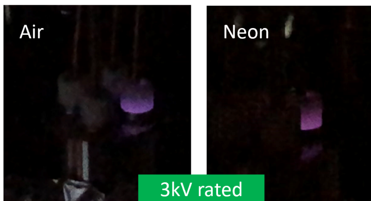
Figure F.3: Arcing on the RF MOT coil electrical feedthrough.
