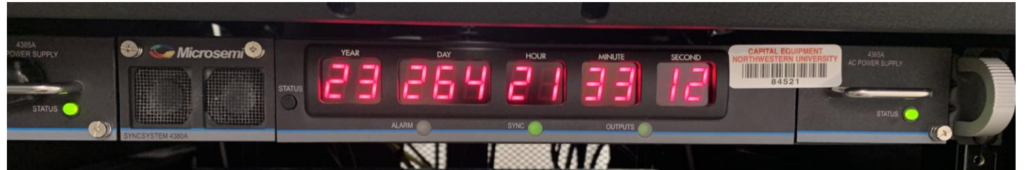
GPS-steered rubidium clock
